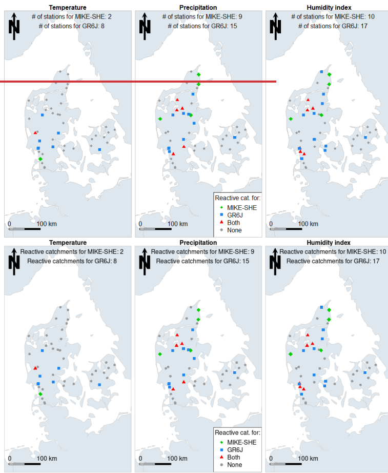
480 Figure 11: Location and number of Danish catchments on which MIKE SHE and GR6J react to the RAT using temperature (left), 485 precipitation (centre) and humidity index (right) as predictors. Numbers at the top of the maps represent the number of reactive catchments out of 43 for each model.
