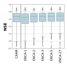
**Figure 3.** NSE values for the considered models in the test period. The boxes are delimited by the 25 % and the 75 % quantiles, while the whiskers indicate to the 5 % and 95 % quantiles. CAAM performance is similar to ENCA-2.
