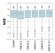
**Figure 3.** NSE values for the considered models in the test period. The boxes are delimited by the 25 % and the 75 % quantiles, while the whiskers indicate to the 5 % and 95 % quantiles. CAAM performance is similar to ENCA-2.
