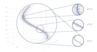
Figure 2. Unidimensional line embedded in three dimensions. The estimated intrinsic dimension depends on the distance scale.
