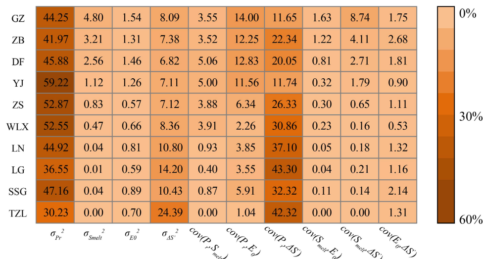
Figure 8. Relative contribution matrix of how variances in different water balance terms ( \sigma_{Pr}^2 , \sigma_{Smelt}^2 , \sigma_{E0}^2 , and \sigma_{\Delta S'}^2 ) and the covariances cov(P, S_{melt}) , cov(P, \Delta S') , cov(P, E_0) , cov(S_{melt}, \Delta S') , cov(S_{melt}, E_0) , and cov(E_0, \Delta S') contribute to runoff variance ( \sigma_R^2 ) during the period 2002-2016 in all sub-basins. The colors indicate the degree of contribution.
