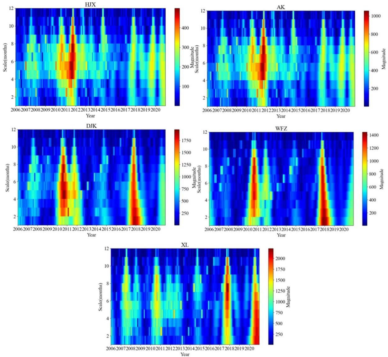
Fig.1. Wavelet transform analysis of runoff for HJX, AK, DJK, WFZ, and XL dam sites.
