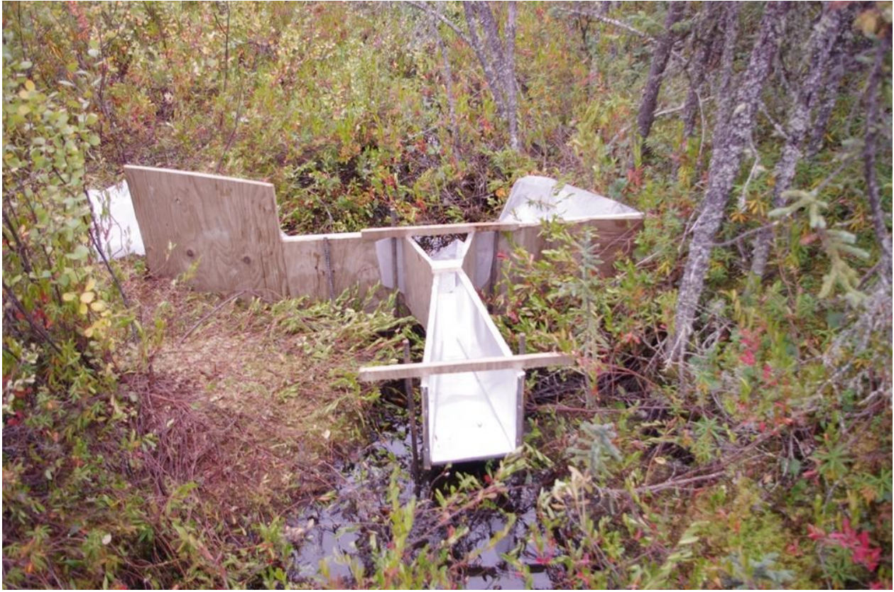
Figure S2. One of the two flume box systems installed at the South sub-basin (the southern one).
