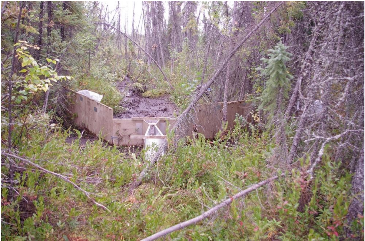
Figure S1. One of the two flume box systems installed at the West sub-basin (the western outlet).
