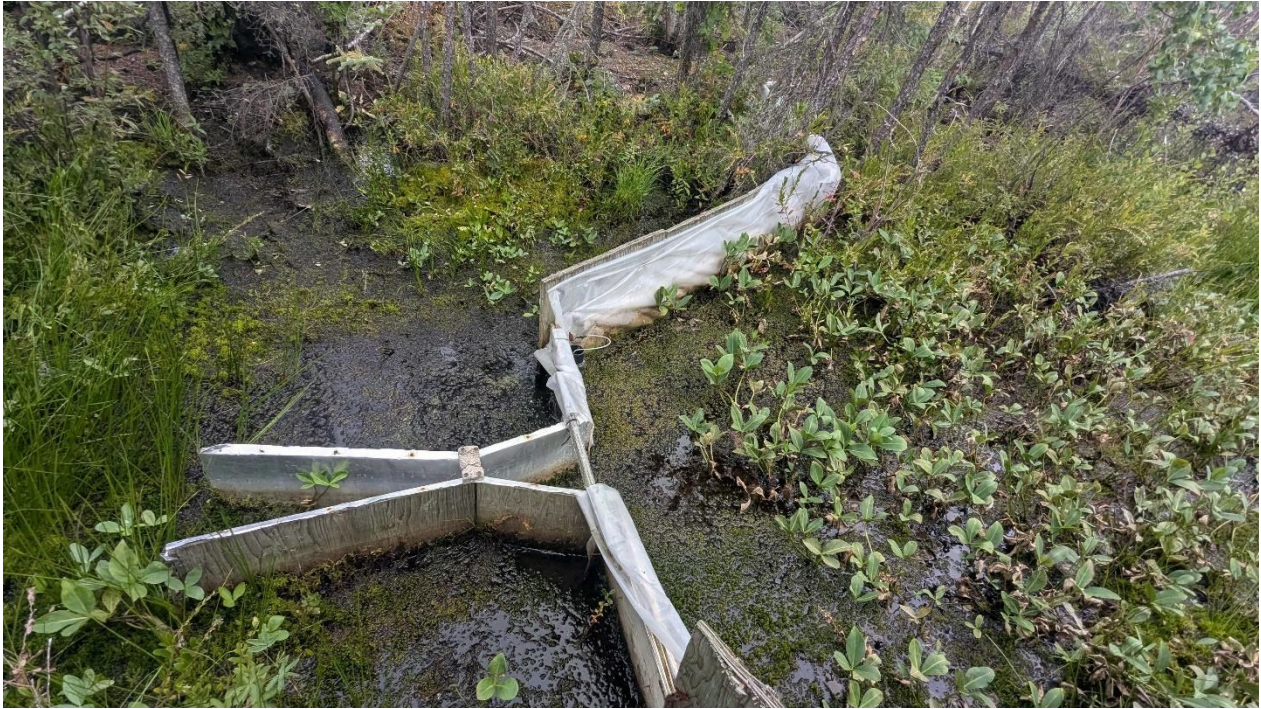
Figure S4: One flume box in August 2024 (post-fire picture).
