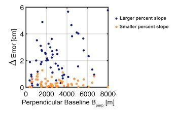
Figure 14. Line-of-sight (LOS) errors (in cm) of all interferogram pairs vs. perpendicular baseline (in m) at  $P_E$ - $P_W$  with percent slopes 8.4% to 11.0% (blue dots) and around  $P_f$  with percent slopes 2.0% to 1.8% (orange dots). The location of these pixels is shown in Figure 10.
