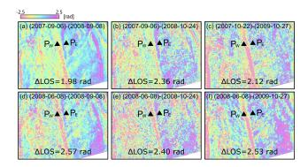
Figure 11. InSAR phase measurements over the zoomed-in region outlined with the black box in Figure 10 for interferograms with large pixel misregistration errors.  $P_E$  and  $P_W$  are on the east-facing and west-facing slopes. Here all interferograms were referenced to a local reference point near  $P_E$ .
