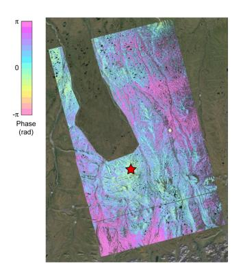
**Figure A1.** An L-band ALOS PALSAR interferogram (Path 255 Frame 1370-1380) that spans June 3, 2006 and July 27, 2009 over the study area. A phase cycle  $(2\pi)$  equals 12 cm radar Line-Of-Sight (LOS) deformation. Subsidence leads to positive LOS deformation (pink). The same reference point at  $68.83^{\circ}$  N,  $150.23^{\circ}$  W were used for both frames, as marked by the red star.
