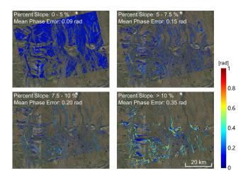
Figure 13. Estimated InSAR phase errors (in radians) at pixels with different slopes (0-5%, 5-7.5%, 7.5-10%, and > 10%). Here DEM errors are introduced by 1 pixel misregistration ( $\sim 12 \text{ m}$ ) to the east as in Figure 12(a). InSAR phase errors were calculated based on an InSAR perpendicular baseline of 5104 m. An error of 1 radian equals an LOS error of 1.9 cm for L-band ALOS data.
