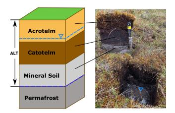
**Figure 4.** (Left) A cartoon showing the three soil layers. The lighter blue dashed line denotes the groundwater level, and the darker blue line shows the location of the permafrost table note that the depth of permafrost may be in any soil layer. (Right) A photo of a soil pit with three soil layers from top to bottom: the acrotelm (peat that contains living plants), the catotelm (peat that contains dead plant materials), and the mineral soil.
