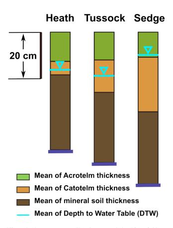
**Figure E1.** Soil stratigraphy under different land covers near Toolik Lake area as derived from field measurements collected at sites marked in Figure 1 in the main paper (Adapted from Chen et al. (2020)).
