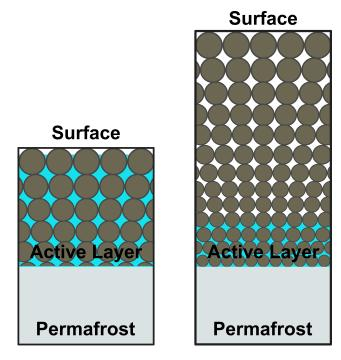
**Figure 2.** (Left) a nearly-saturated soil column with a shallower active layer. (Right) a relatively dry soil column with a thicker active layer. Because the left soil column stores more soil water in the active layer, we expect to observe more thaw subsidence over this soil column.
