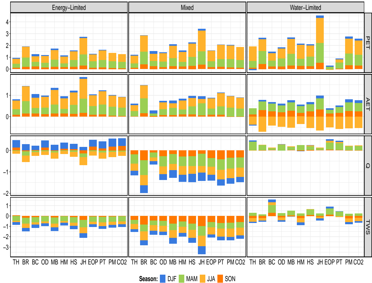
Figure S12. Seasonal trend contribution in annual trend for each catchment category for PET and all the hydrological components (AET, Q, and TWS). Abbreviations used for hydrological cycle components are as follows: PET, AET, Q and, TWS represent potential evapotranspiration, actual evapotranspiration, runoff and, total water storage, respectively. Abbreviations used for different PET methods are TH: Thornthwaite, BR: Bair-Robertson, BC: Blaney-Criddle, OD: Oudin, MB: McGuinness-Borden, HM: Hamon, HS: Hargreaves-Samani, JH: Jensen-Haise, MD: Milly-Dunne, PT: Priestley-Taylor, PM: Penman-Monteith, CO 2 : Modified Penman-Monteith accounts CO 2 . For seasons DJF, MAM, JJA, and SON indicate summer, spring, summer, and autumn, respectively. Y-axis units are in mm/seas/year.
