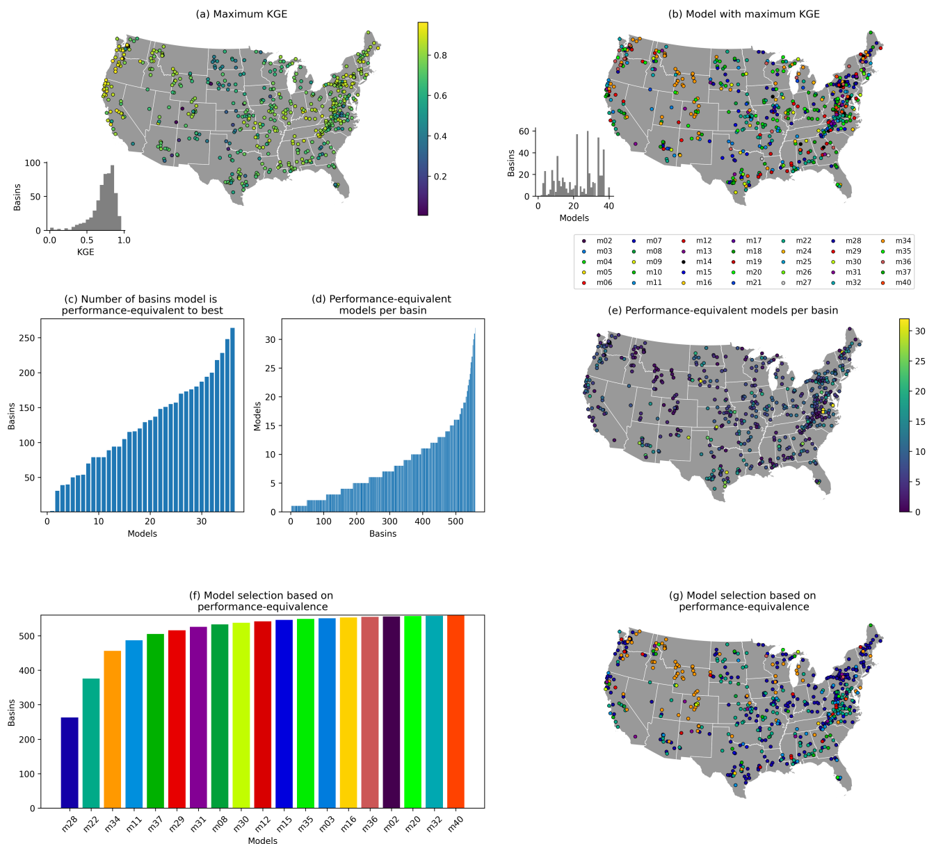
Figure 5. Repeat of earlier analysis for models calibrated with a KGE(1/Q) objective function. (a) Maximum KGE score per basin. (b) Model from which the maximum KGE score in each basin is obtained. (c) Number of times each model falls within the uncertainty bounds around the performance of the best model in each basin. Note that a model can fall within its own uncertainty bounds. (d) Number of models that fall within the uncertainty bounds around the best model’s performance for each basin. (e) Spatial overview of [d]. (f) Number of basins covered by an increasing number of models. m xx refers to the model identifier. (g) Spatial distribution of basins covered by each model (colors refer to specific models as shown in (f)).
