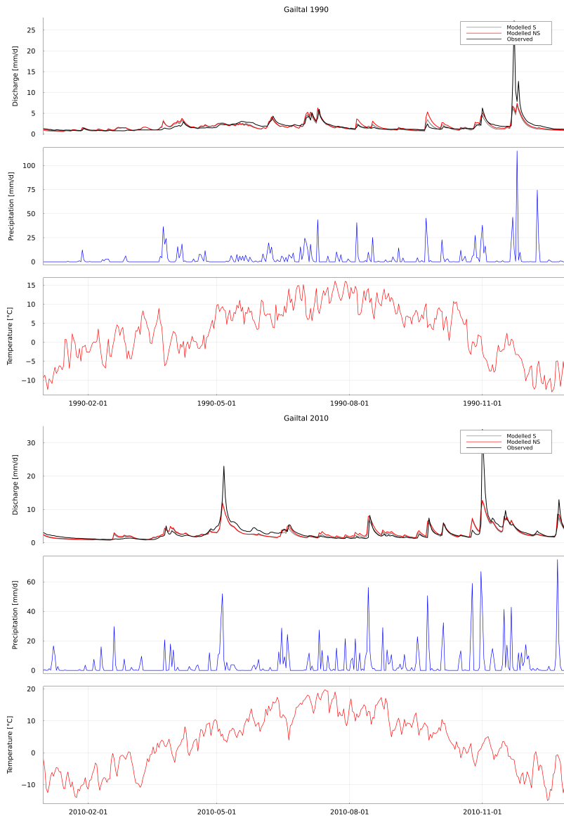
Fig. S9. Comparison of measured and both calibrated and climate-based modelled runoff in the Gaital, also showing the corresponding temperature and precipitation. The solid lines indicate mean modelled runoff using the best parameter sets, shaded areas show the range of best parameter sets
