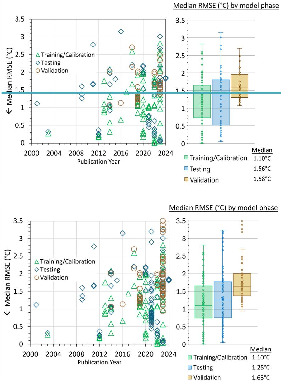
**Figure 4. Median RMSE (°C) values from published literature for training/calibration, testing, and validation phases of model evaluation.**
