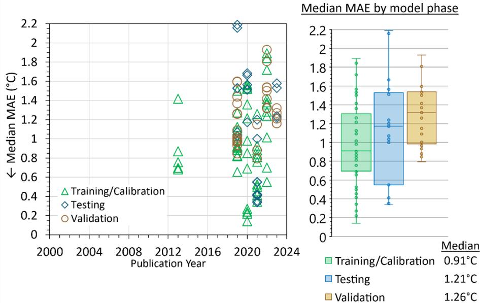
750 **Figure 5. Median MAE (°C) values from published literature for training/calibration, testing, and validation phases of model evaluation.**
