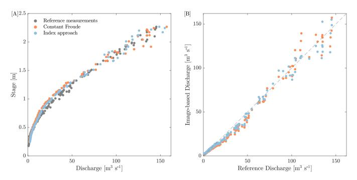
**Figure 8.** [A] Stage-discharge plots for the River Dart at Austins Bridge (UK) following analysis of imagery acquired over a one-year period (shown in the red and blue), and developed using conventional flow gauging techniques between 1981-2018 (grey). [B] Comparison between image-based discharge estimates and reference discharge estimates with 1:1 line shown.
