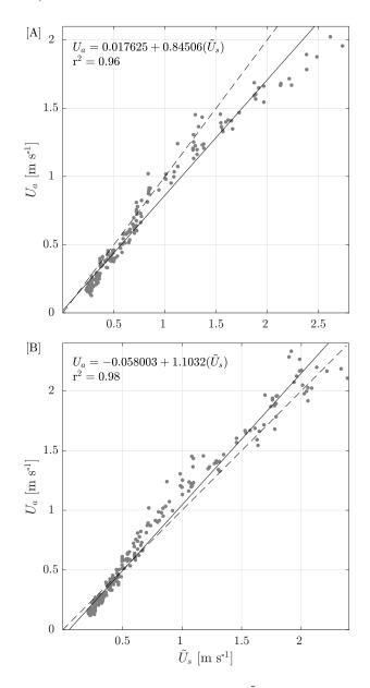
**Figure 7.** Bi-plot and linear fit between KLT-IV derived velocity measurements  $[\tilde{U}_a]$  and reference velocity measurements  $[U_a]$  during [A] the calibration period and [B] validation period. The solid line represents the linear fit between variables, with the 1:1 line also shown (dashed line).
