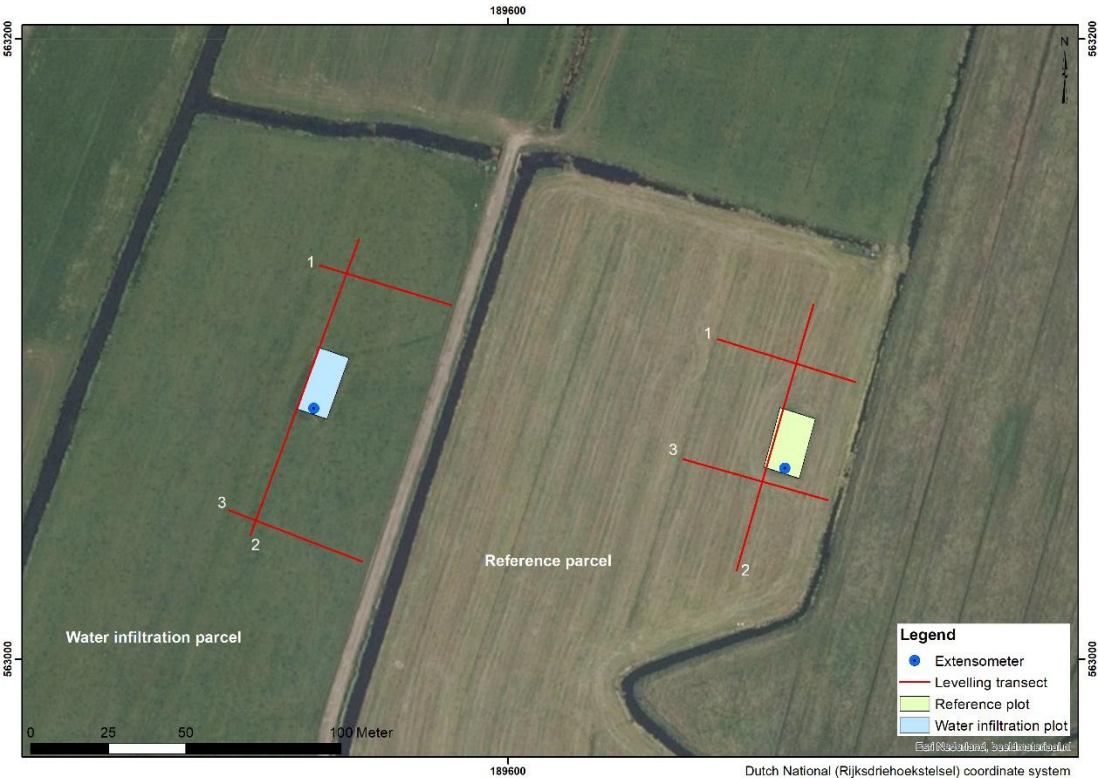
Figure 4. Position of field plots, spirit levelling transects and extensometers in the reference and PWIS parcel at Aldeboarn.
