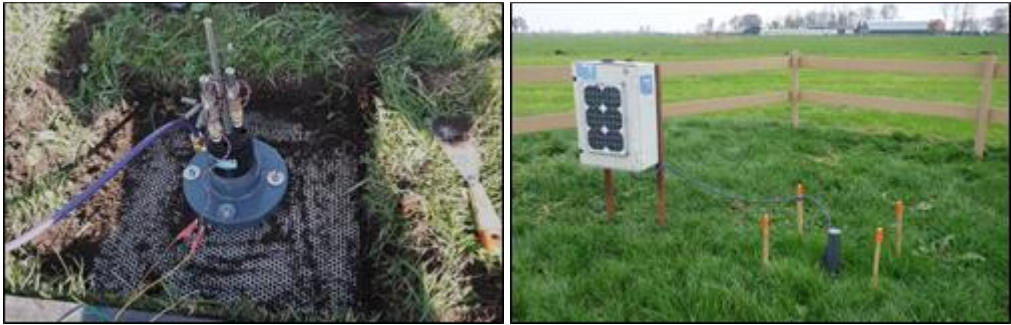
Figure 3. Left: extensometer head and stainless-steel plate a few centimetres below surface level. Right: extensometer protected by a PVC cover and connected to the datalogger with solar panels.
