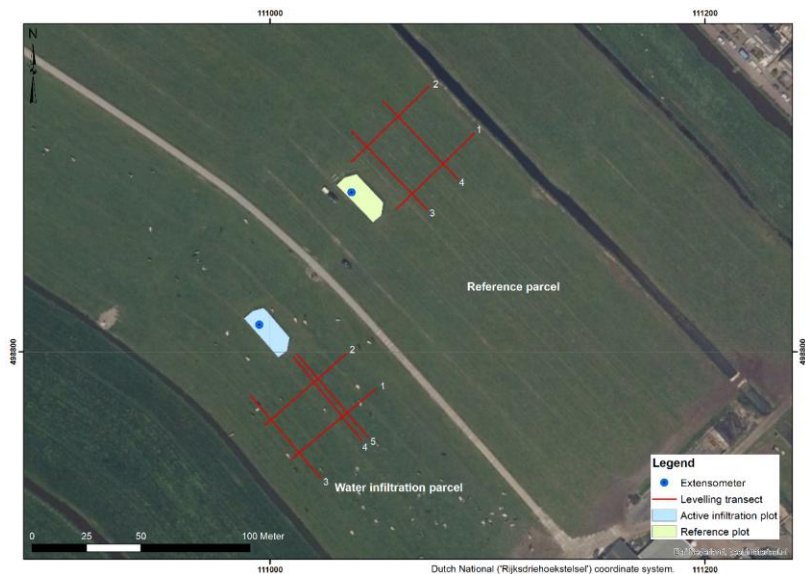
Figure 6. Position of field plots, spirit levelling transects and extensometers in the reference and AWIS parcel at Assendelft.
