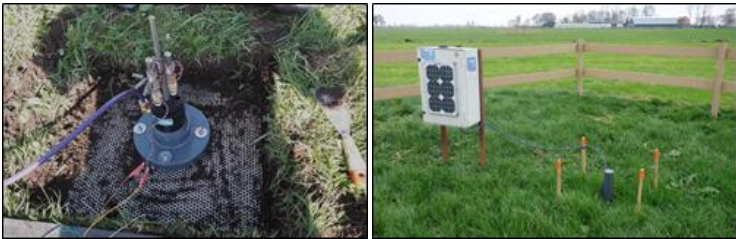
Figure 3. Left: extensometer head and stainless-steel plate a few centimetres below surface level. Right: extensometer protected by a PVC cover and connected to the datalogger with solar panels.
