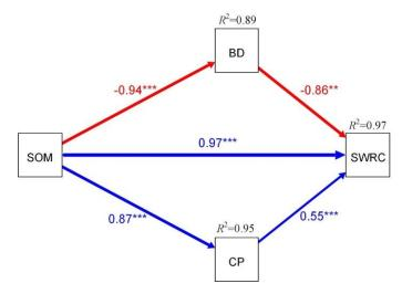
Fig. 8 Structural equation modeling of the direct and indirect effects of soil properties on soil water retention capacity (SWRC) among two surface soil types. Standardized path coefficients, adjacent to arrows, are analogous to partial correlation coefficients, and indicative of the effect size of the relationship. Continuous blue and red lines represent positive and negative correlations, respectively. Model fit: Fisher.C=5.48, df=2, P-value=0.065.
