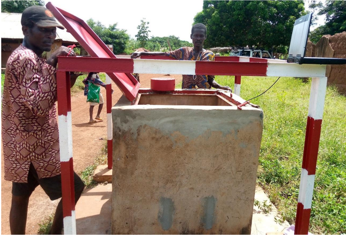
Piezometric level measurements in the field
