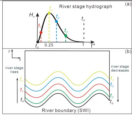
**Figure 1.** (a) River stage hydrograph during the flood event; (b) diagram showing displacement of SWI during the flood event. The colored SWIs in (b) correspond to the times of colored dots in (a). When the river stage increases, the river boundary migrates into the aquifer and recovers to its initial location as river stage decreases as also indicated by the arrows.
