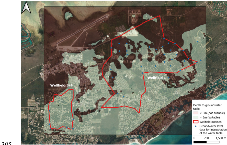
305 Figure 4. MAR suitability map with respect to the depth to the groundwater table, for the populated areas of Wellfields 1, 3 and 4 (source of base map: © Google Maps)
