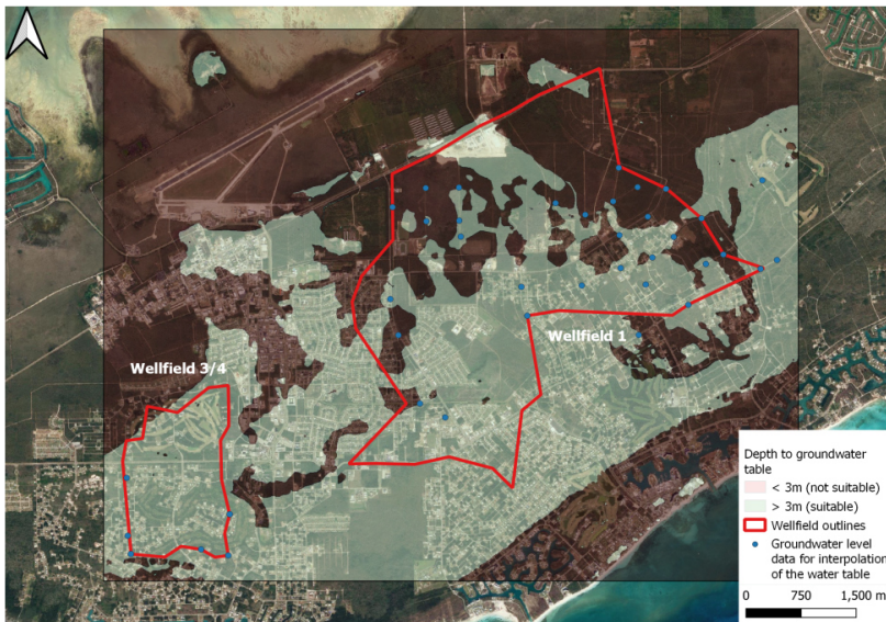
Figure 4. MAR suitability map with respect to the depth to the groundwater table, for the populated areas of Wellfields 1, 3 and 4 (source of base map: © Google Maps)
