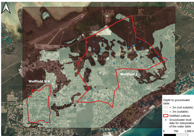
310 Figure 4. MAR suitability map with respect to the depth to the groundwater table, for the populated areas of Wellfields 1, 3 and 4 (source of base map: © Google Maps)
