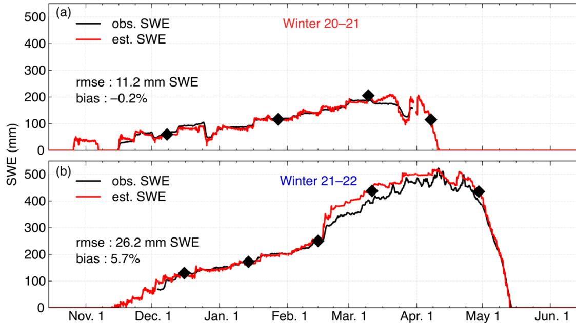
50 Figure S5: Comparison between the SWE monitored by the CS725 and the SWE derived from density profiles interpolation and snow height measurement in NEIGE site. The RMSE corresponds to 5.9% of the maximum SWE in winter 2020–21 and to 5.0% of the max SWE in winter 2021–22. Black diamonds show the corresponding date of the density profile measurements.
