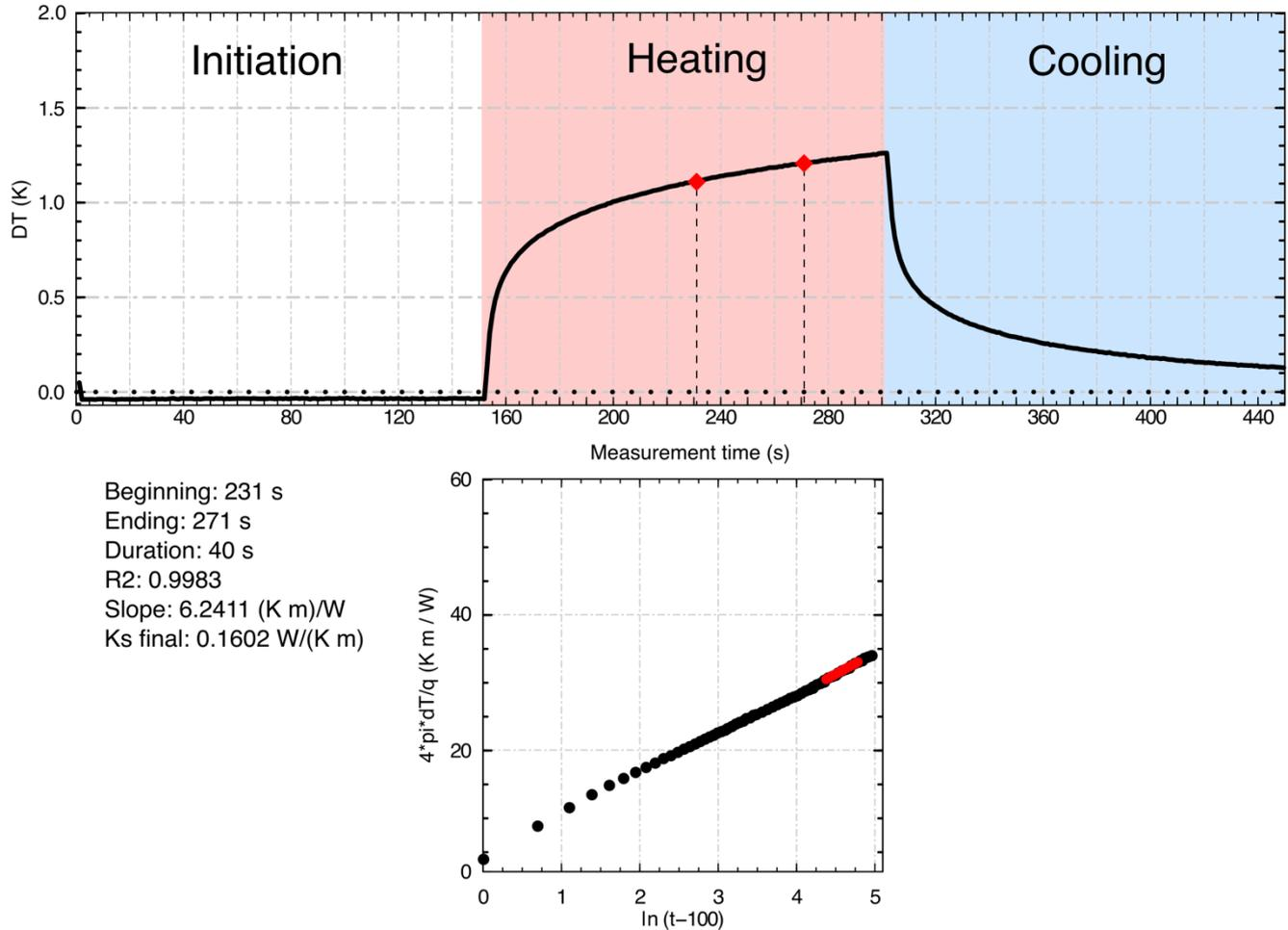
15 **Figure S1: Heating curve analysis for the 80-cm needle from the monitoring station in the medium gap on 2 February 2022. In this example, we selected a period of 40 seconds that started at 231 seconds. The slope is 6.24 K m W<sup>-1</sup> which gives a  $k_s$  of 0.16 W m<sup>-1</sup> K<sup>-1</sup>. Since  $R^2$  is greater than 0.98 and no convection was detected, the measurement is considered valid.**
