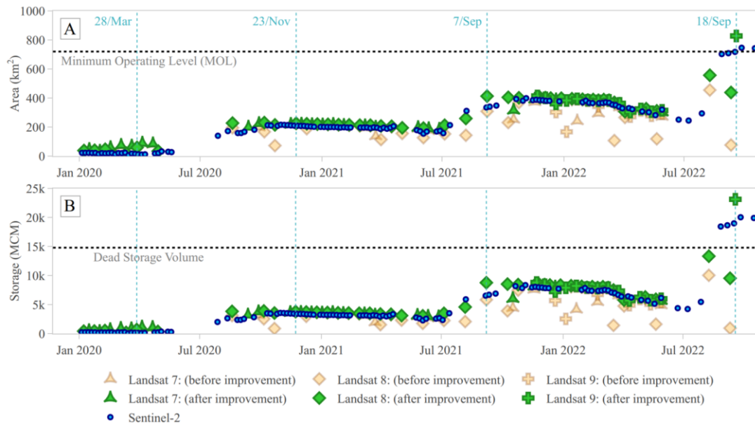
Figure 6. Satellite-derived GERD reservoir information during the filling period 2020 - 2022. Panel (A) shows the derived water surface area while panel (B) shows the derived storage volume of GERD using Landsat (Green: before improvement; Light orange: after improvement) and Sentinel (blue). The WSA maps of the dates specified in cyan dotted lines are illustrated in Fig. 7. Note that not filling the gaps induced by the Scan Line failure of Landsat 7 produces NDWI = 0 in these gaps when using the algorithm of Vu et al. (2022). Therefore, in case of negative NDWI thresholds (which were the case here), Landsat 7 overestimates the areas and storages.
