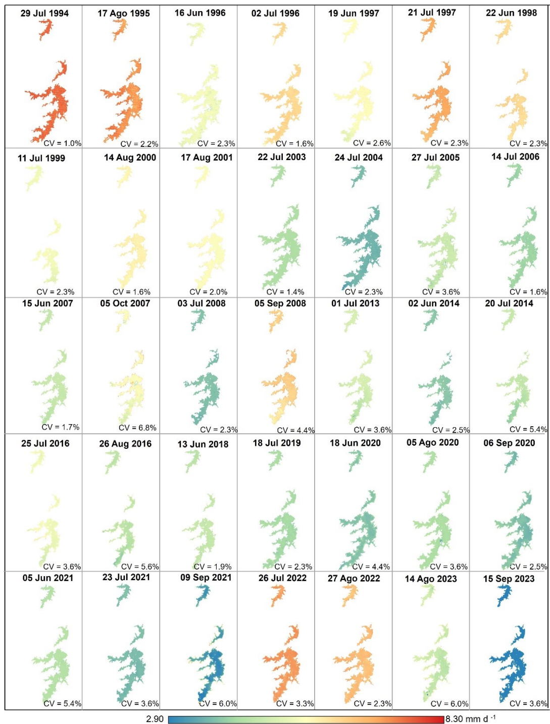
240 Figure 4: Evaporation rates in the Fortaleza Metropolitan Region reservoirs (Gavião, Riachão and Pacoti) obtained with AquaSEBS algorithm for 35 individual days in the period 1994-2023.
