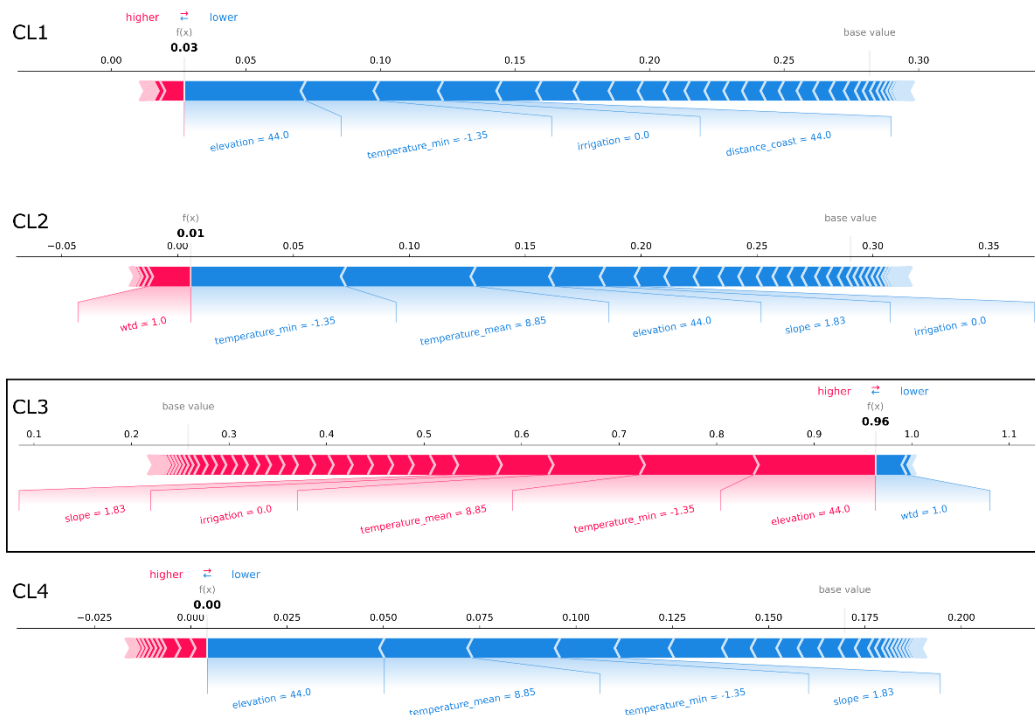
625 Figure E6 SHAP force plots explaining the correct prediction of the CL3 exemplary well site from the case study region in northern Germany (Fig. 5a) (from top to bottom: CL1, CL2, CL3, and CL4). At this well site, the probability that CL3 is predicted is the largest in the case study (test dataset). The average scores of all classifications made by the Random Forest model for the training dataset are 0.28, 0.29, 0.26, and 0.17 respectively (base values). The model's probability scores for predicting the clusters at the exemplary well site (bold printed numbers) sum up to 100%. Features that are important for the respective predictions are displayed 630 with their values. Their importance and effects can be assessed by the SHAP values visualized by bar length and color (i.e. the larger the feature's share of the bar the more important; red represents rejecting effect and blue represents supporting effect).
