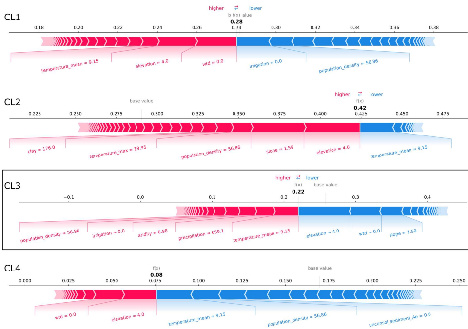
Figure E5 SHAP force plots explaining the prediction of the CL3 exemplary well site from the case study region in northern Germany (Fig. 5a) (from top to bottom: CL1, CL2, CL3, and CL4) that is confused with CL2. At this well site, the probability that CL2 is predicted is the largest in the case study (test dataset). The average scores of all classifications made by the Random Forest model for the training dataset are 0.28, 0.29, 0.26, and 0.17 respectively (base values). The model's probability scores for predicting the clusters at the exemplary well site (bold printed numbers) sum up to 100%. Features that are important for the respective predictions are displayed with their values. Their importance and effect can be assessed by the SHAP values visualized by bar length and color (i.e. the larger the feature's share of the bar the more important; red represents rejecting effect and blue represents supporting effect).
