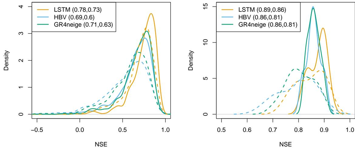
**Figure 2.** Overview of NSE values of all modelling approaches for the calibration period (solid) and the validation period (dashed) for all 668 basins (left) and for the 12 basins selected for metamorphic testing (right; note the different scale of the x-axis). The median NSE values are indicated in brackets in the legend (calibration period, validation period).
