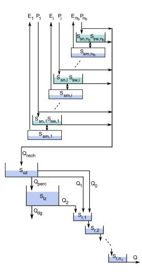
Figure A4. Schematic diagram of the HBV model as used in this paper.
