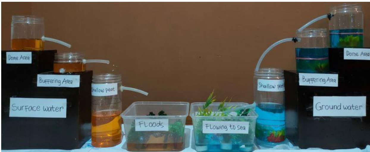
670 Figure D3. Simple water balance model of the H 2 Ours game in Pawan-Kepulu peatland to show the dynamics of changes in hydrological conditions as a result of the changes in land-use and canal density. The red line in each tank in the groundwater system represent the fire vulnerable threshold.
