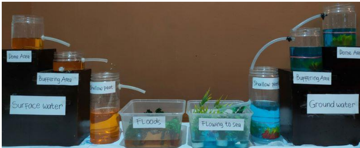
660 Figure D3. Simple water balance model of H 2 Ours game in Pawan-Kepulu peatland to show the dynamics of changes in hydrological conditions as a result of the changes in land-use and canal density. The red line in each tank in the groundwater system represent the fire vulnerable threshold.
