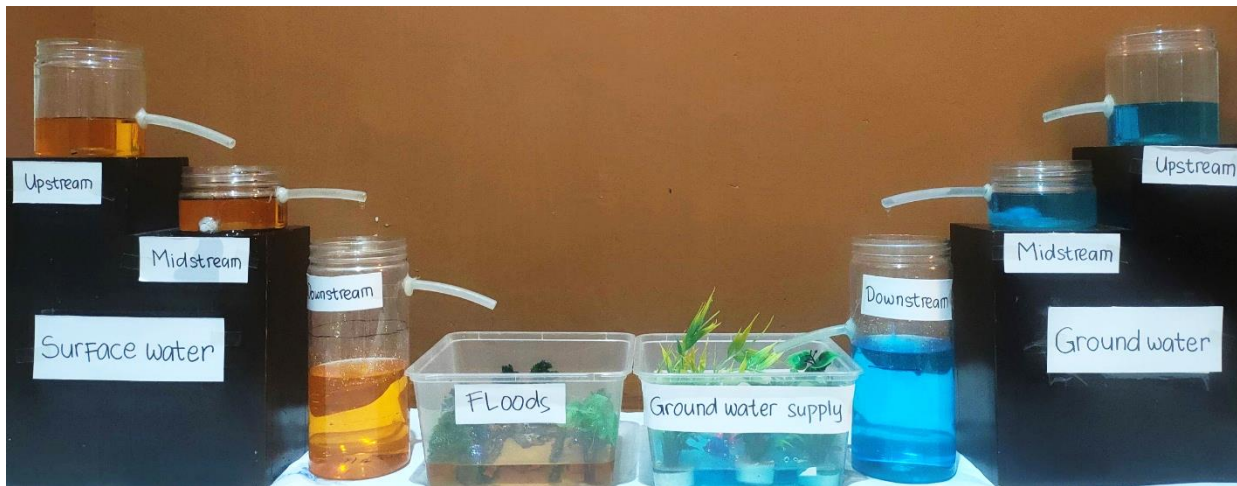
380 Figure 6: Simple water balance model of H 2 Ours game in Rejoso watershed to show the dynamics of changes in hydrological conditions because of land-use change and water utilization. See appendix D for the simple water balance model for the Pawan-Kepulu peatland
