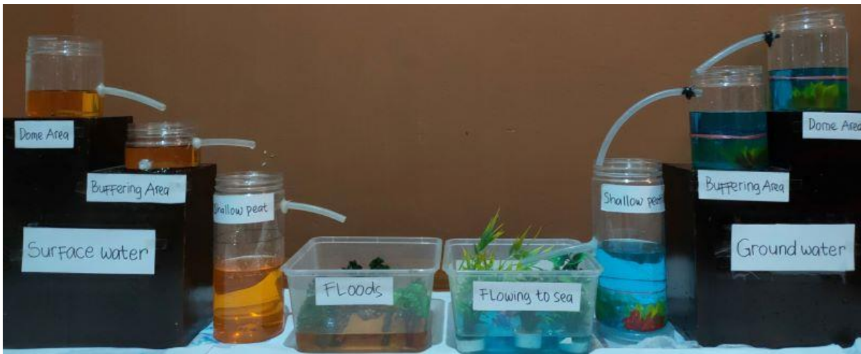
630 Figure D3. Simple water balance model of H 2 Ours game in Pawan-Kepulu peatland to show the dynamics of changes in hydrological conditions as a result of the changes in land-use and canal density. The red line in each tank in the groundwater system represent the fire vulnerable threshold.
