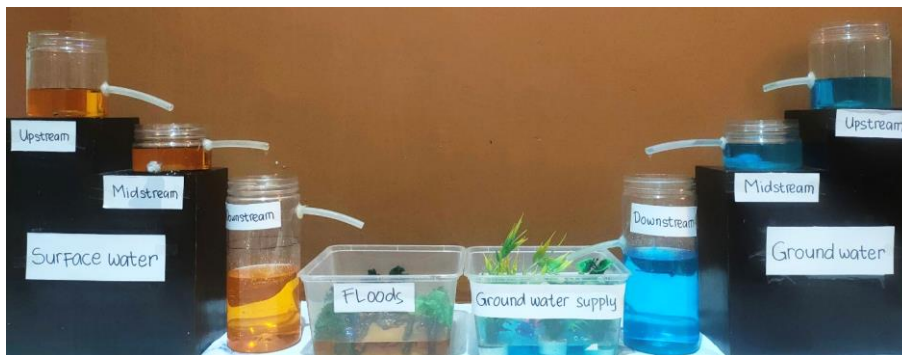
425 Figure 6: Simple water balance model of H 2 Ours game in Rejoso watershed to show the dynamics of changes in hydrological conditions because of land-use change and water utilization. See appendix D for the simple water balance model for the Pawan-Kepulu peatland
