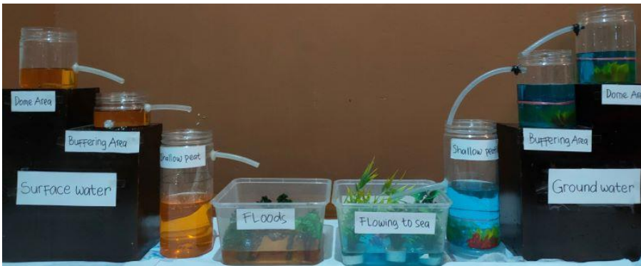
690 Figure D3. Simple water balance model of H 2 Ours game in Pawan-Kepulu peatland to show the dynamics of changes in hydrological conditions as a result of the changes in land-use and canal density. The red line in each tank in the groundwater system represent the fire vulnerable threshold.
