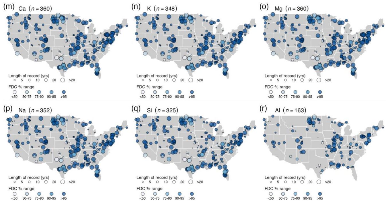
Figure 6: Range of the flow duration curve (FDC %, symbol color) and length of record (symbol size) for the stream data between 1980 and 2018 for (a) discharge, (b) dissolved oxygen (DO), (c) pH (field), (d) temperature, (e) dissolved organic carbon (DOC), (f) total organic carbon (TOC), (g) dissolved organic nitrogen (DON), (h) total organic nitrogen (TON), (i) total dissolved nitrogen (TDN), (j) nitrate ( \text{NO}_3 ), (k) Cl, (l) bicarbonate ( \text{HCO}_3 ), (m) sulfate ( \text{SO}_4 ), (n) Ca, (o) K, (p) Mg, (q) Na, (r) Si, and (s) Al. The inset histogram shows the number of samples by 8-year periods. Note: we do not show alkalinity or DIC here because coverage is so limited in the dataset (Table 2).
