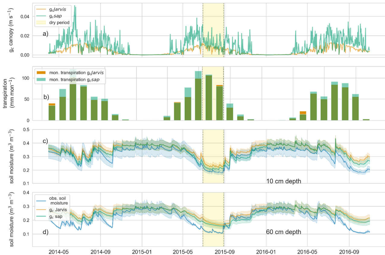
275 Figure 3. a) daily averaged canopy conductance estimates for g_{c,sap} (green) and g_{c,Jarvis} (orange); b) monthly transpiration sums estimated using g_{c,sap} (green) and g_{c,Jarvis} (orange); observed (blue) and simulated soil moisture \pm standard deviation of the corresponding simulation and observations ( g_{c,sap} : green; g_{c,Jarvis} : orange) at 10 (c) and 60 cm depth (d). Highlighted in yellow is a dry period from July to August 2015.
