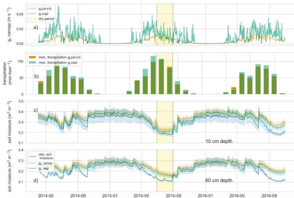
280 Figure 3. a) daily averaged canopy conductance estimates for g_{sap} (green) and g_{Jarvis} (orange); b) monthly transpiration sums estimated using g_{sap} (green) and g_{Jarvis} (orange); observed (blue) and simulated soil moisture \pm standard deviation of the corresponding simulation and observations ( g_{sap} : green; g_{Jarvis} : orange) at 10 (c) and 60 cm depth (d). Highlighted in yellow is a dry period from July to August 2015.
