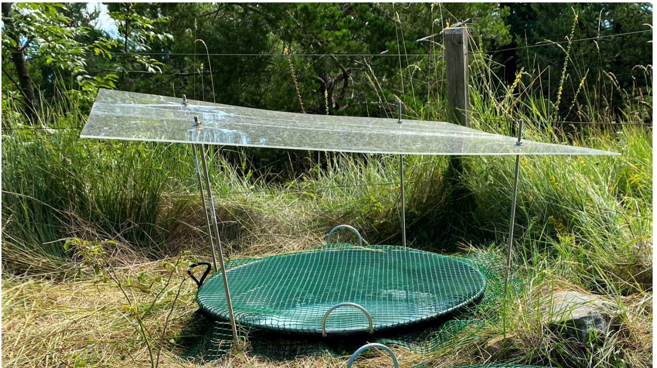
Figure 1: View of steel experimental pan. The pan was partly buried in the ground and protected against precipitation by a lid of clear methacrylate installed 0.5 m above the pan surface, to allow air circulation, and against large animals drinking by a net.
