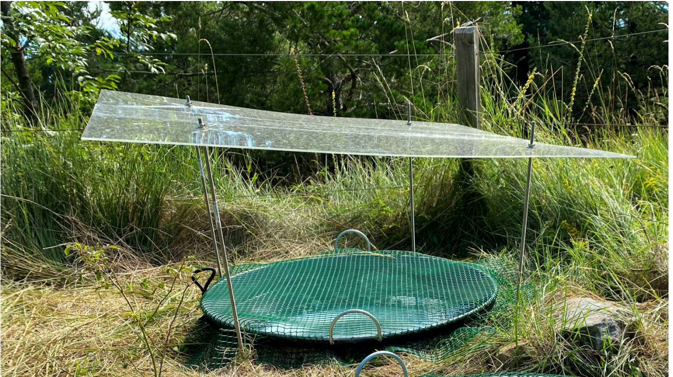
Figure 1: View of steel experimental pan. The pan was partly buried in the ground and protected against precipitation by a lid of clear methacrylate installed 0.5 m above the pan surface, to allow air circulation, and against large animals drinking by a net.
