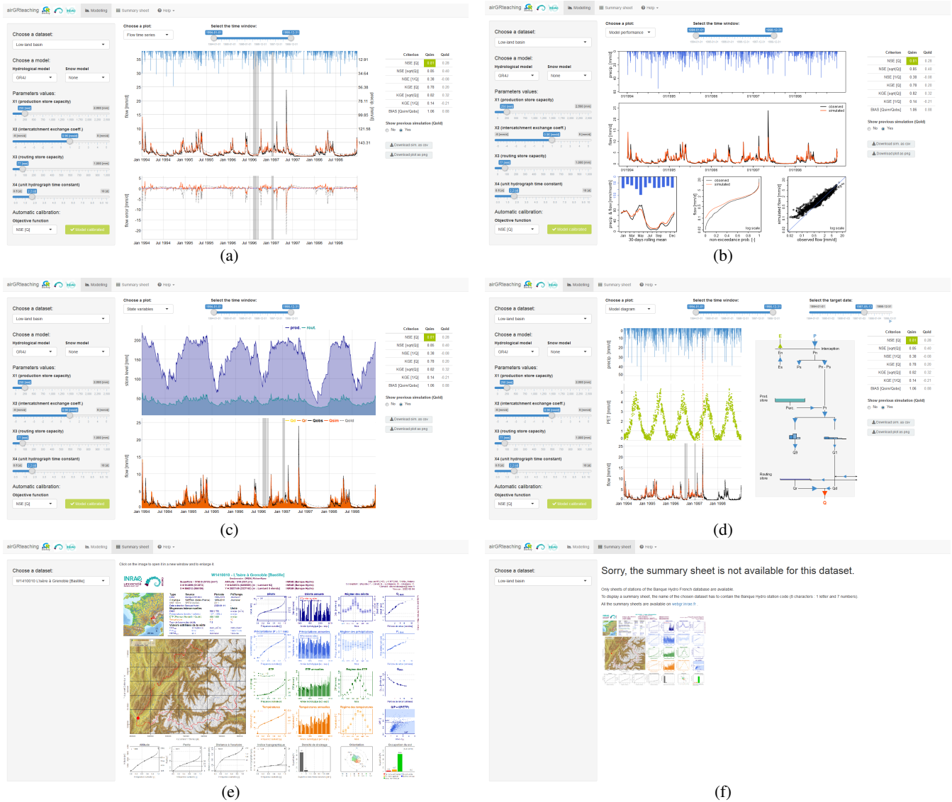
Figure 2. airGRteaching GUI "Modeling" panels (a-d) and "Summary sheet" panels (e-f) that can be reached through diverse clicking. In the following, the center column of the GUI is described for each possible panel; all other elements of the GUI were described in Fig. 1. (a) "Flow time series": precipitation, observed and simulated hydrographs (top), and flow error time series (bottom). (b) "Model performance": precipitation (top), observed and simulated hydrographs (middle), simulated and observed regime hydrographs (bottom left), flow duration curves (bottom center), and a scatter plot between simulated and observed discharges (bottom right). (c) "State variables": time series of reservoir levels (top) and runoff components (bottom). (d) "Model diagram": time series (left) of precipitation, potential evapotranspiration, simulated and observed flows (from top to bottom), and interactive model diagram (right; with updating of the flows, the size and the level of the reservoirs). (e) Hydrometeorological and topographical characteristics of the selected catchment (Brigode et al., 2020, only available for French catchments). (f) Same as (e) when the catchment characteristics are not available.
