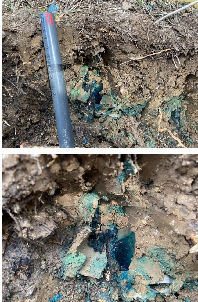
Figure S3. Dye colored water observed at mini-piezometer wt-W20, located next to the west TDR probe (30 cm distance from tree trunk; swc-W30).
