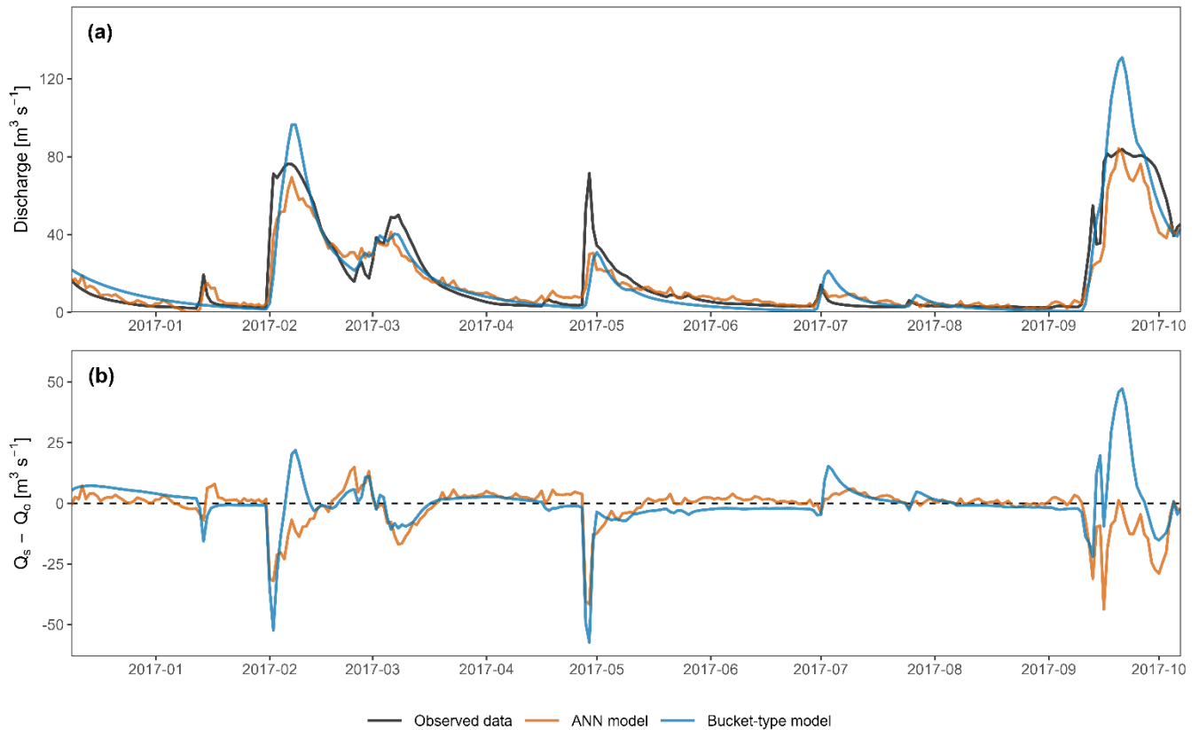
Figure 6: (a) Observed and simulated spring discharge time series on the validation period. (b) Relative difference between simulated and observed discharge on the validation period.
