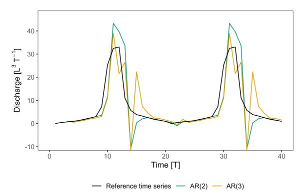
Note that, the synthetic time series of the example hydrograph has no value before t = 0, therefore the first three values of the autoregressive projections will be non-defined as  $Q_{obs}(t-1)$ ,  $Q_{obs}(t-2)$  and  $Q_{obs}(t-3)$  are NA. Because of this, we evaluated the models on the whole synthetic time series except the first three values, as can be appreciated on the graph below:
