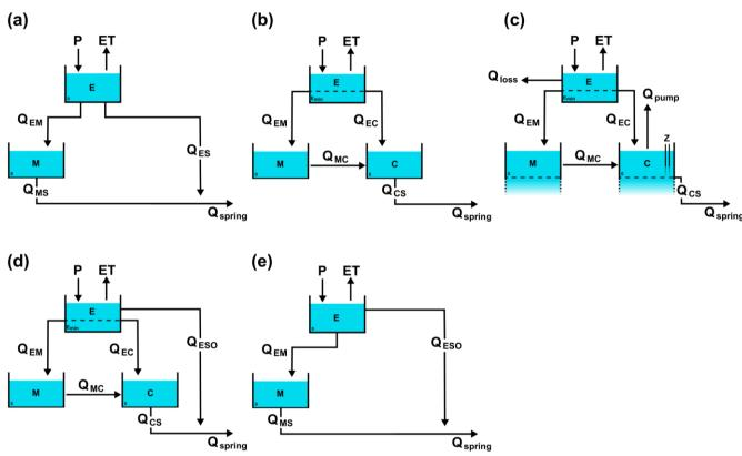
255 Figure 3: Selected model structures for (a) Aubach, (b) Gato Cave, (c) Lez, (d) Qachqouch and (e) Unica springs. Flux names correspond to the terminology of the KarstMod platform (Mazzilli and Bertin, 2019).
