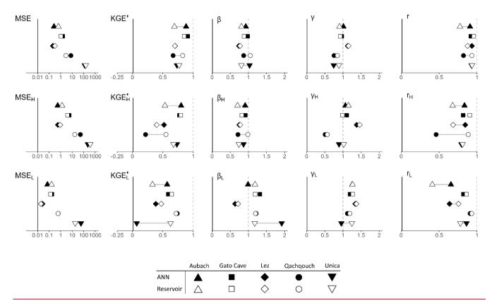
Figure 46: Performance of the ANN and reservoir models on the validation period, according to different performance criteria. Exact values can be found in Table 4.
