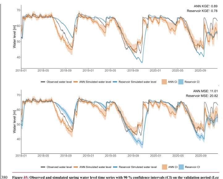
Figure 35: Observed and simulated spring water level time series with 90 % confidence intervals (CI) on the validation period (Lez spring).
