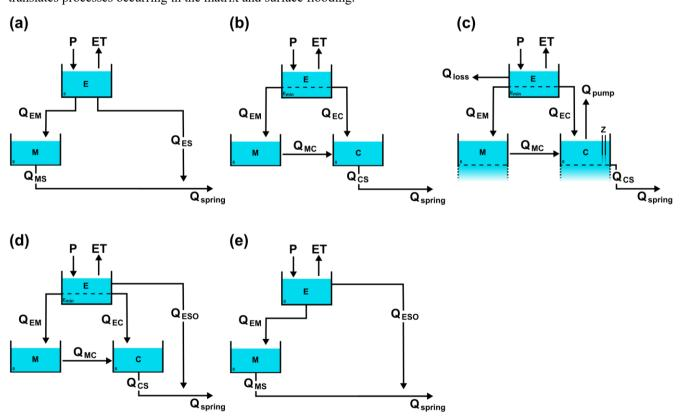
Figure 43: Selected model structures for (a) Aubach, (b) Gato Cave, (c) Lez, (d) Qachqouch and (e) Unica springs. Flux names correspond to the terminology of the KarstMod platform (Mazzilli and Bertin, 2019).
