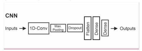
Figure 2: Selected structure of the CNN model.
