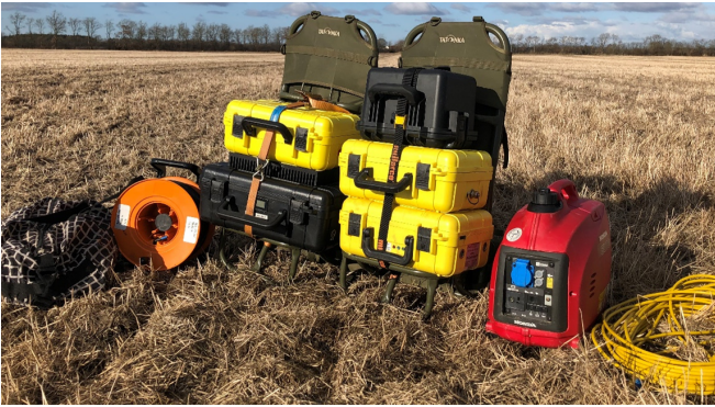
Figure 1. The Apsu SNMR instrument, mounted on two backpacks carried by a two person crew.
