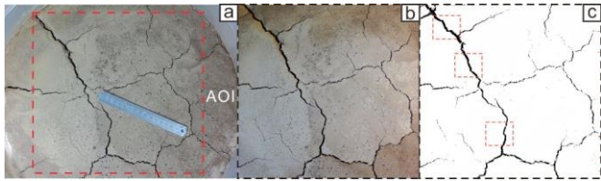
156 157 Fig. 3 Process of crack image processing. (a) a photo obtained from the HD camera, 800 pixels × 1400 pixels; (b) crack 158 image after cropping and pixel enhancement, 1044 pixels × 1005 pixels; (c) crack image after binarization and denoise, and 159 the crack ratio was calculated as the crack area divided by the overall area of interest, the crack aperture was calculated as the 160 average value of crack aperture from three different positions.
