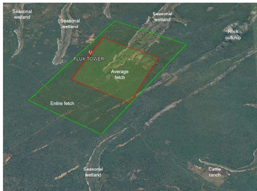
910 Figure A1. Analysis of the wind direction and wind speed using the wind rose (a) and the extent of the fetch for the DTS observations (b) based on the wind rose results.
