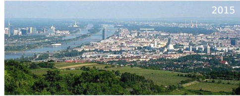
315 Figure 10. Long term human-flood interactions illustrated for the Danube at Vienna, Austria. In 1830 the river near Vienna was braided. As a consequence of devastating floods, a cut through channel was constructed in 1870, as seen in the 1930 photo. The enhanced protection triggered urban development on the flood plain, which required an additional relief channel constructed in 1970, which eventually led to further urban development. The attempt of increasing protection has thus increased rather than reduced the damage potential. These unintended consequences are studied in socio-hydrology. Barendrecht et al. (2017).
