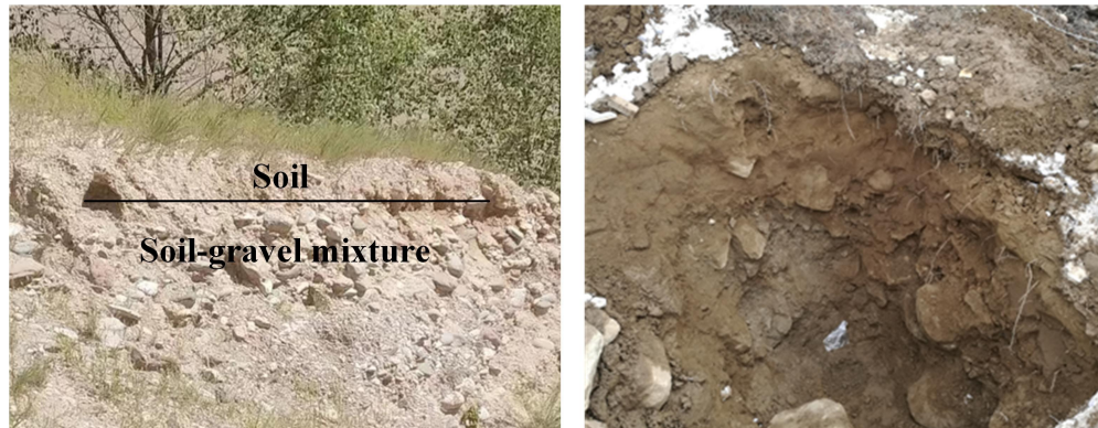
155 Figure 2: Soil and gravel structure of the Niyang River basin (pictures taken near the experimental site labeled in Fig. 1).
