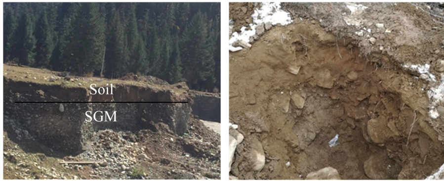
Figure 2: Soil and gravel structure of the Niyang River Basin (pictures taken near the experimental site in Figure 1)
