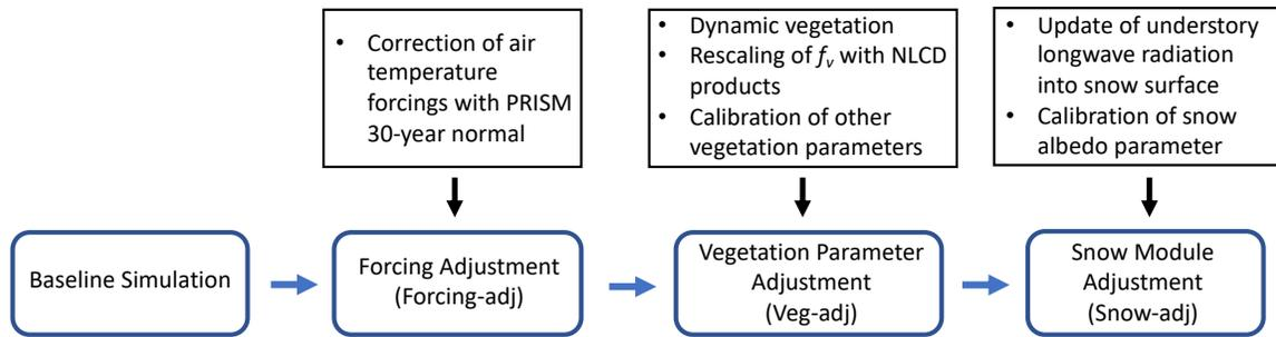
251 **Figure 3.** Flowchart of the stepwise calibration procedure.
