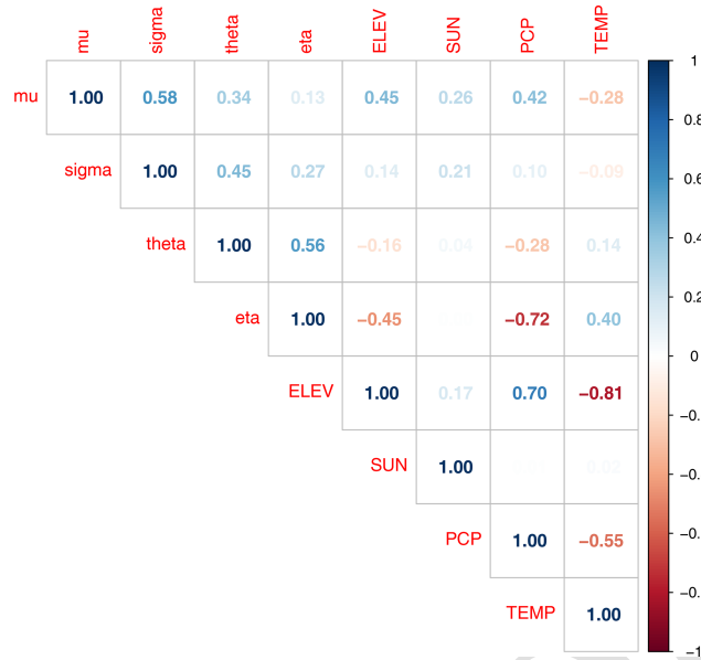
Figure A1. Cross-correlation between the selected local parameters (Koutsoyiannis and GEV parameters) for regionalisation and useful site characteristics that might act as an external drift information. \mu (mu) is the GEV location parameter, \sigma (sigma) the GEV scale parameter, and \theta (theta) and \eta (eta) the Koutsoyiannis parameters. ELEV is short for elevation information, SUN is short for long-term average of annual sunshine duration, PCP is short for long-term average of annual rainfall amount, and TEMP is short for the long-term average of annual mean temperature.
